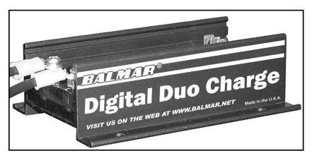
enables the Duo Charge to monitor the ambient temperature of the battery being charged. Should a battery over-temperature condition occur, the Duo Charge will automatically discontinue charging at the battery.
