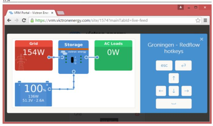
After enabling the feature in the CCGX setting menu, setting or disabling the password, and then restarting the CCGX, a green button will show on the VRM website. Click it to open the Remote Console.
